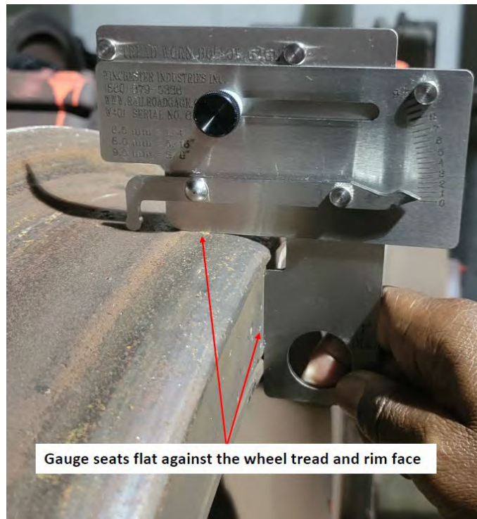
Figure 2. Tread Worn Hollow Gauge positioned Correctly
