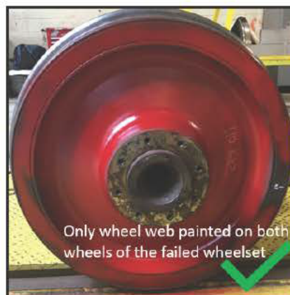
Figure 1. Correct Paint Application on Failed Wheelsets
