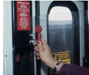
...to break the glass and access the manual door opener.
