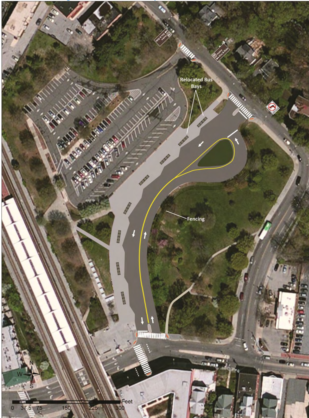
Figure 125: Recommended improvements at Takoma Station
