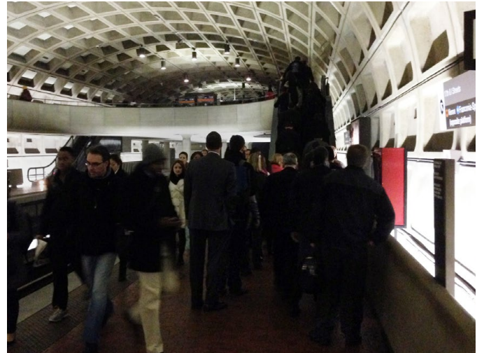
Farragut West queuing at escalator from eastbound platform to East Mezzanine in the AM peak; the pedestrian tunnel would exacerbate congestion without additional vertical circulation capacity
