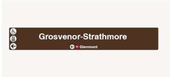
SID Station Identification Sign Located at the platform level, helps passengers confirm they've arrived at the right transfer station
