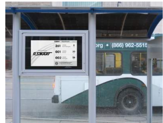
An example of E-ink real-time bus schedule sign at a bus stop.
