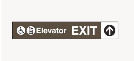
SW1 Station Wayfinding Sign Guides passengers from the platform to the single exit or mezzanine of the station
