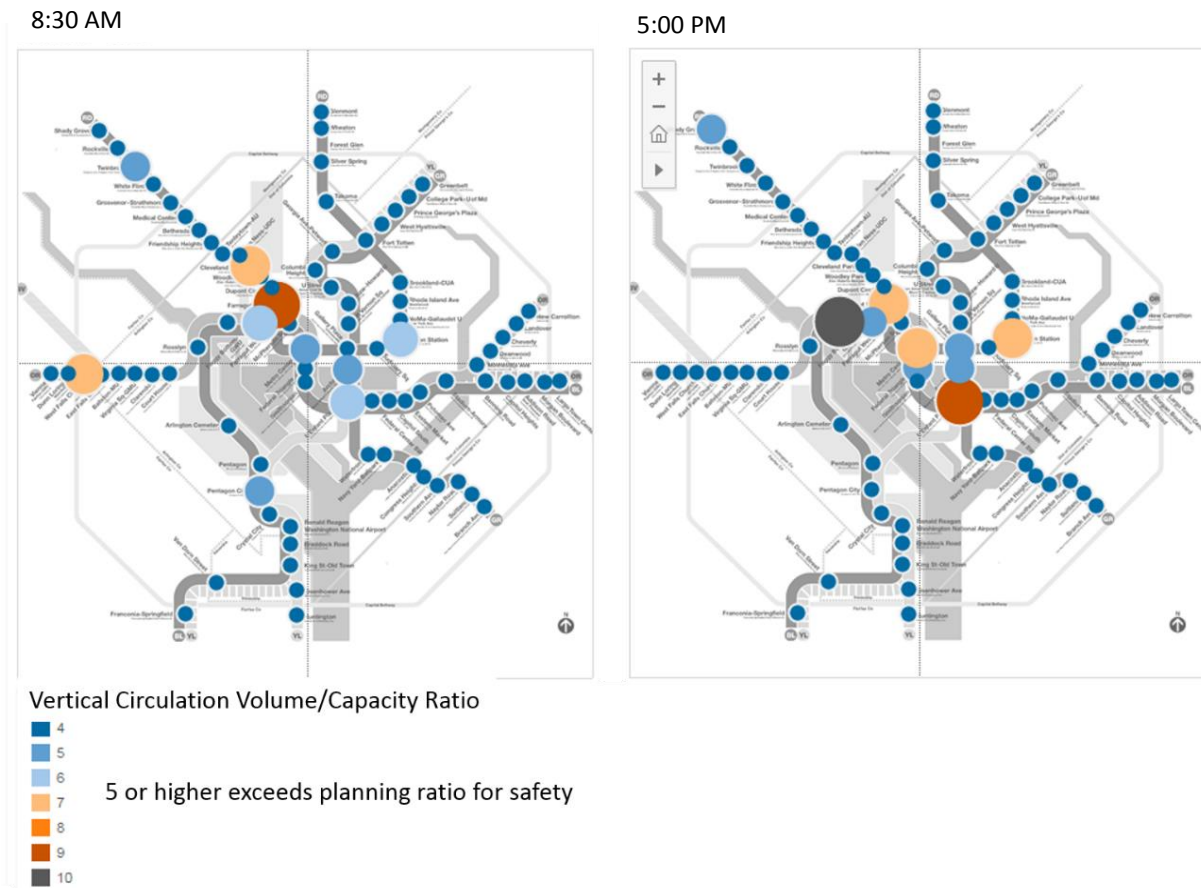
Figure 1: Current Vertical Circulation Capacity Ratio
