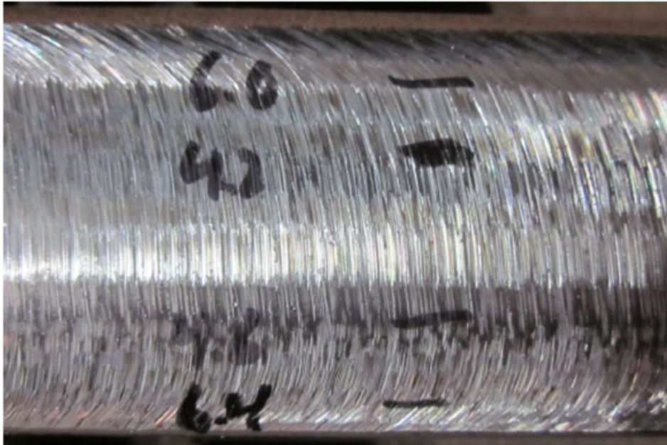
Figure 31 Photograph of left ground rail (guage corner at bottom) ( [REDACTED] "WMATA Post-Grind Surface Roughness Report", Loram Maintenance of Way, December 2013, Figure 1 of Page 2)
