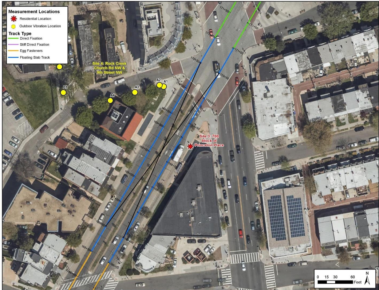
Figure 69: Aerial Map of 700 block of Princeton Place NW Residence and Exterior Measurement Location
