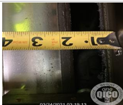
Figure 7: Flangeway Gap Measurement Under tolerance
