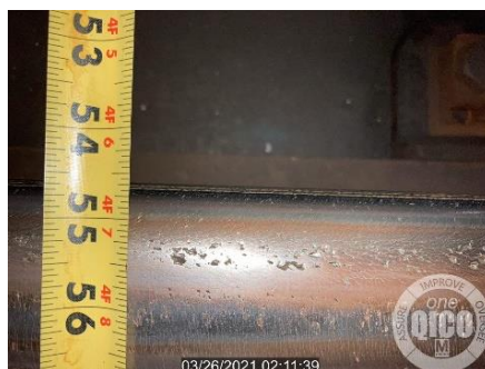
Figure 11: Rail Check Measurement Over Tolerance
