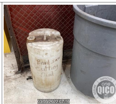
Figure 08: Improperly labeled and stored chemical container
