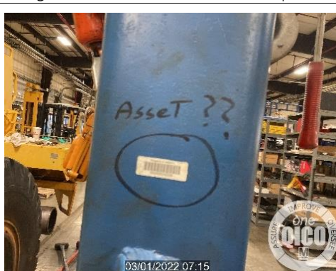
Figure 04: A lifting jack missing asset identification
