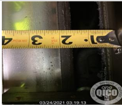
Figure 7: Flangeway Gap Measurement Under tolerance
