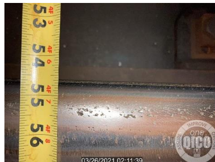
Figure 11: Rail Check Measurement Over Tolerance
