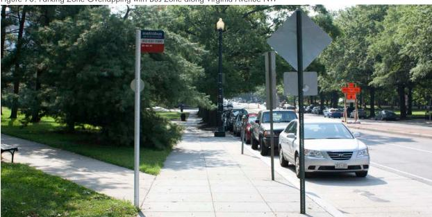
Figure 70: Parking Zone Overlapping with Bus Zone along Virginia Avenue NW
