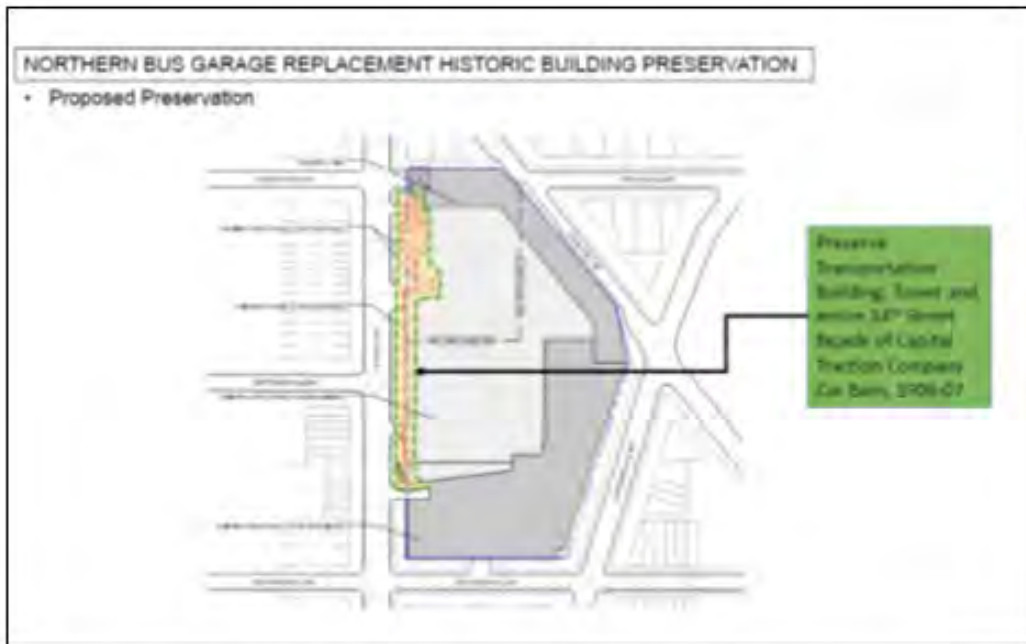
Section of façade for Preservation and Grey Areas for Demolition
