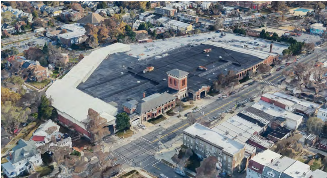
Figure 10. 1987 photograph looking east showing the extent of the demolition that occurred within the bus garage. The entire ceiling and roof structure in this area was removed except for one bay along the perimeter of the east wall (WMATA Archive, George Washington University Special Collections)
