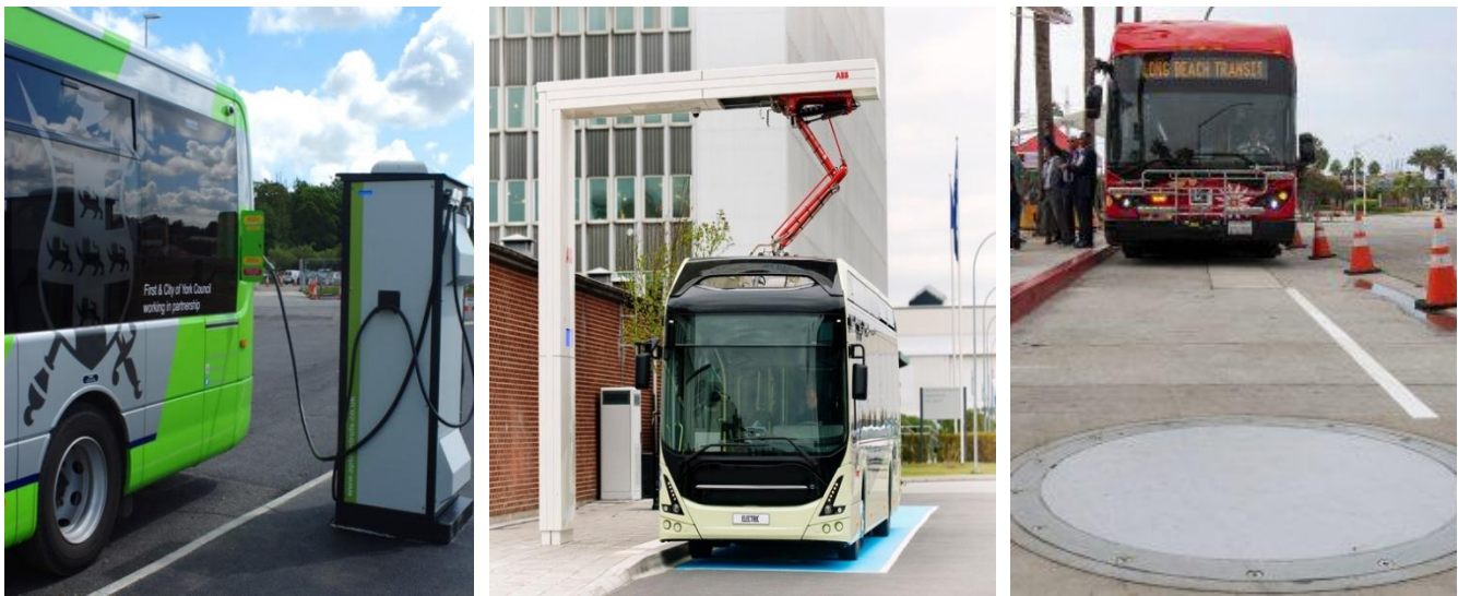
Figure 2-6. Battery-Electric Bus Charging Methods
