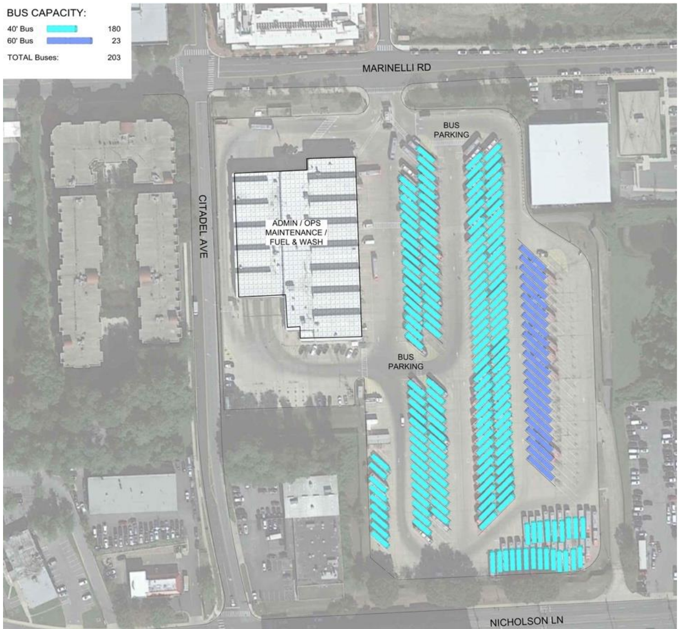
Figure 4-21. Montgomery Garage – Existing Site Layout
