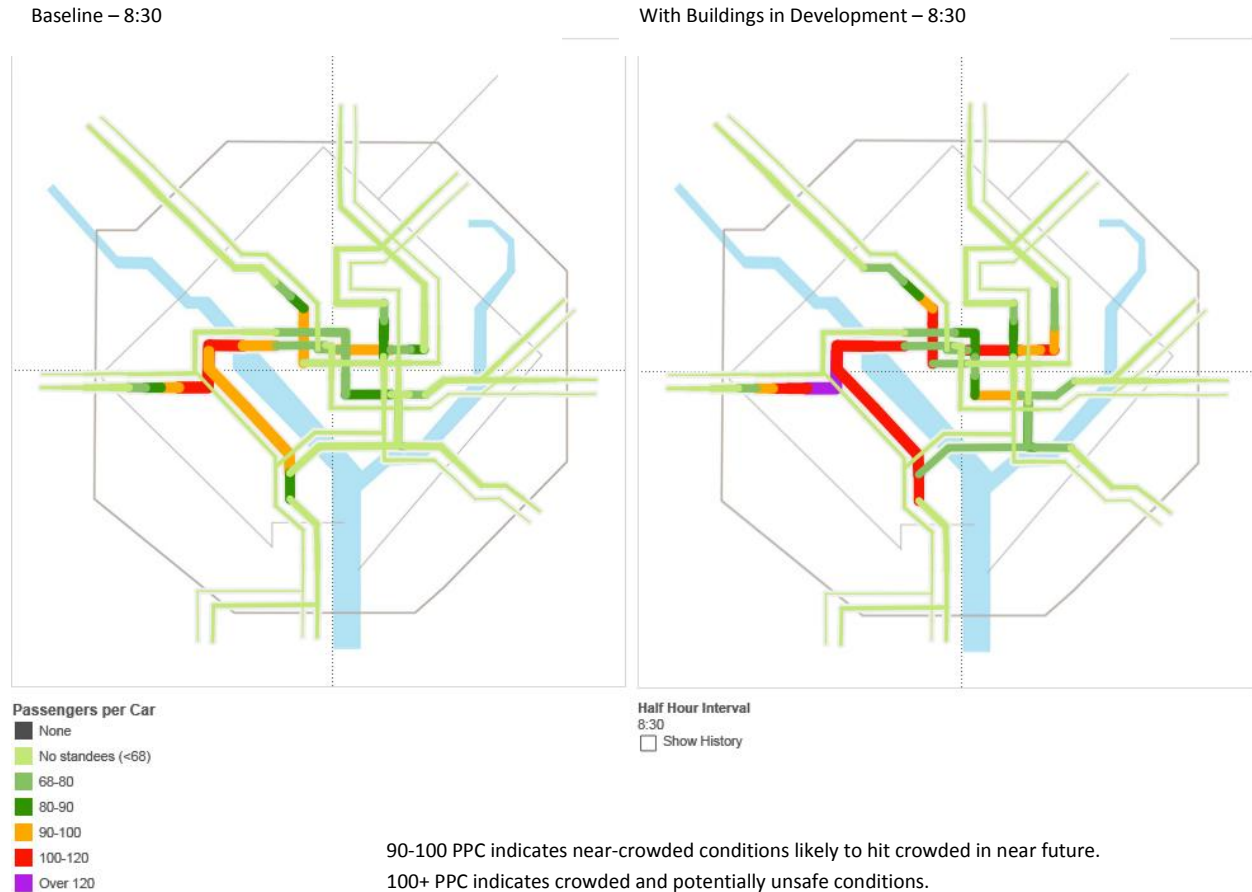
Figure 2: Current Operations Passengers per Car
