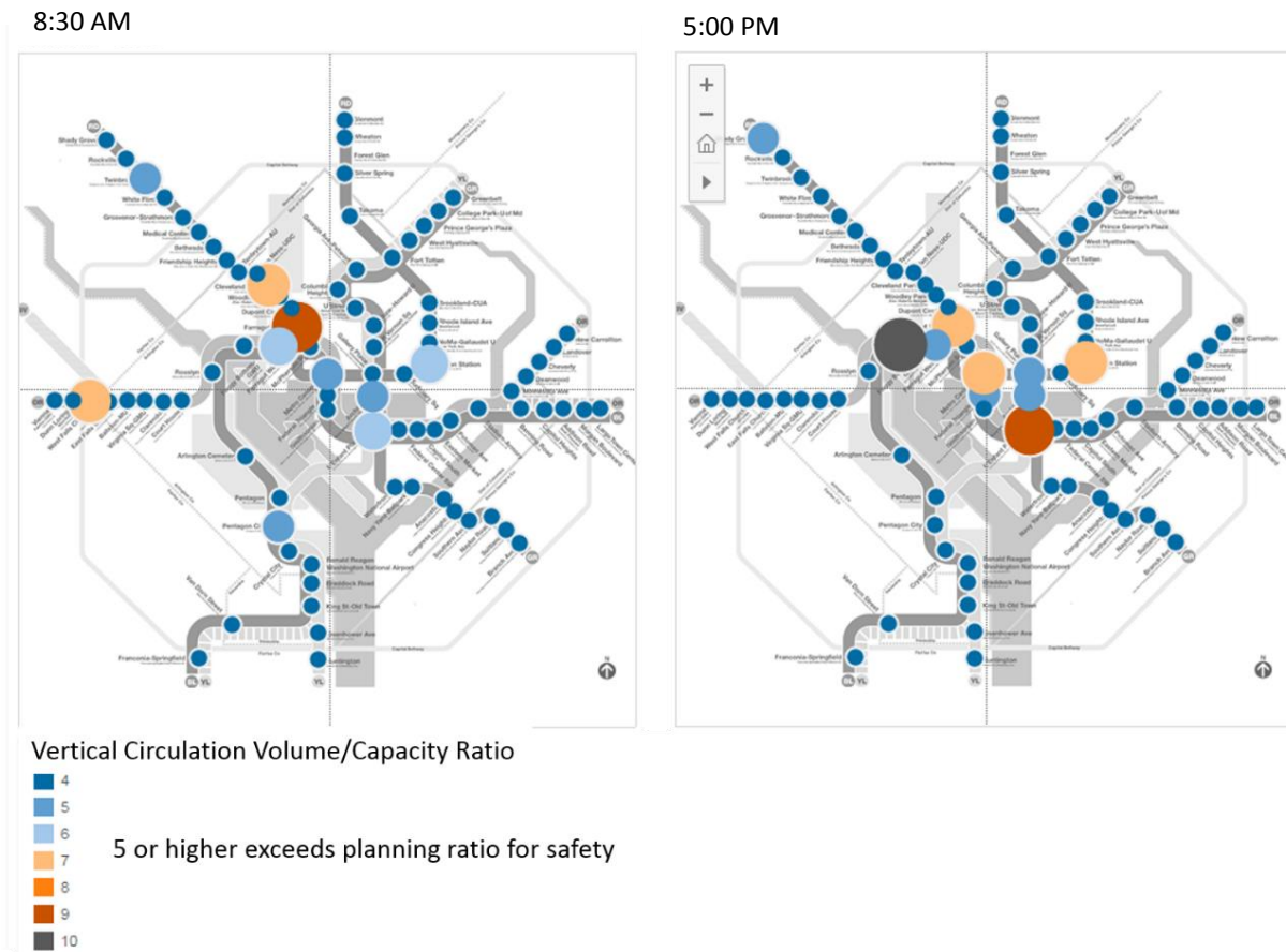
Figure 1: Current Vertical Circulation Capacity Ratio
