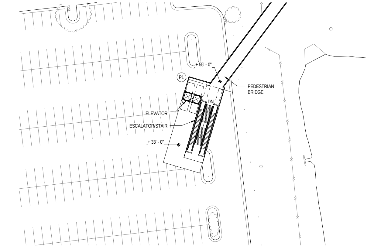
1 NORTH TOUCH-DOWN PLAN AT MEZZANINE LEVEL 1" = 30'-0"
