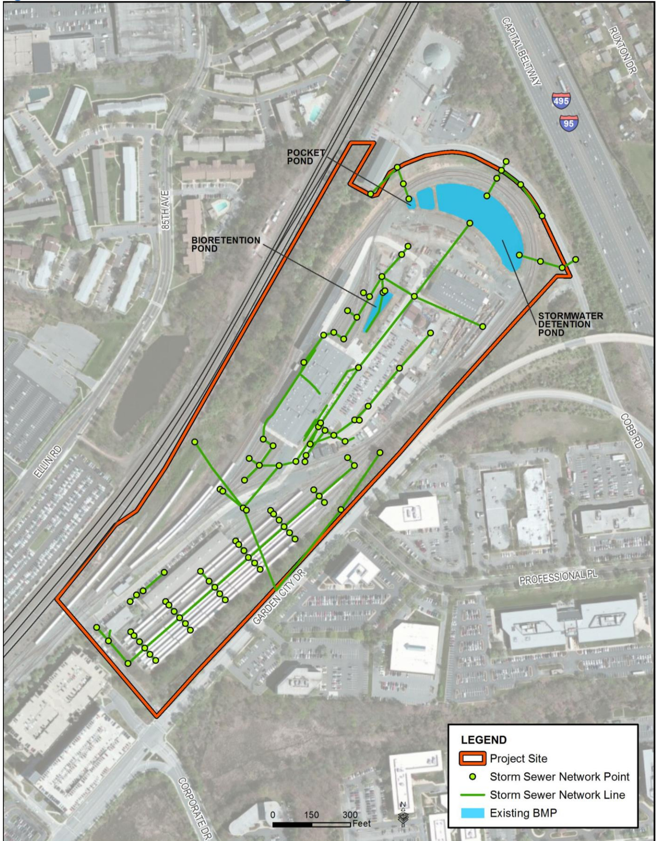
Figure 3-6: New Carrollton Yard Stormwater Management Features
