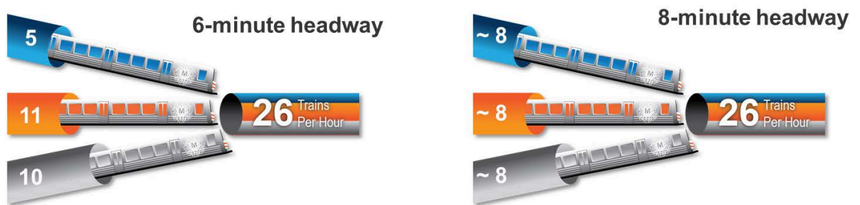
Fig. 2. Maximum Frequencies at the Maximum Capacity (26 TPH)
