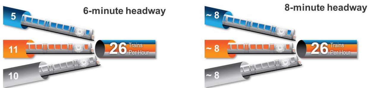
Fig. 2. Maximum Frequencies at the Maximum Capacity (26 TPH)
