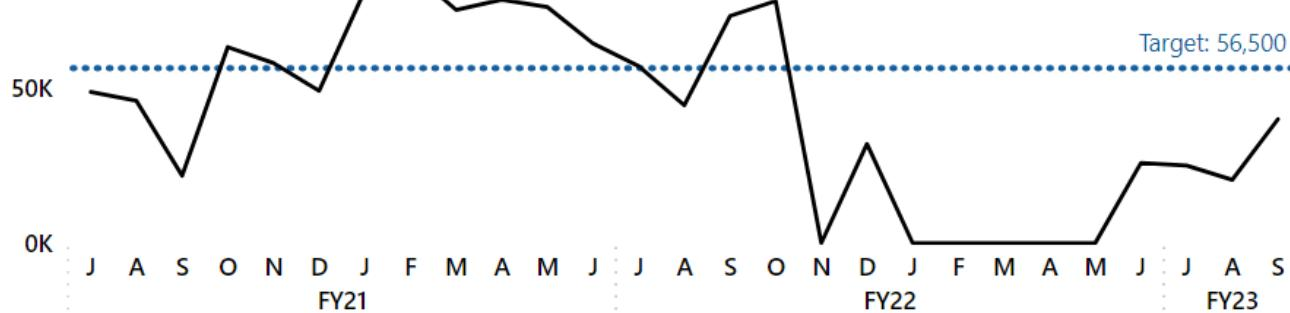
**Chart takeaway** | The 7000-series railcars have traditionally been the most reliable part of Metro's fleet, consistently traveling more than 50,000 miles between failure prior to the derailment of a 7000-series train in October 2021. After briefly returning in December, railcars have steadily run since June and reliability has improved. This trend is expected to continue as more of the fleet returns to service.
