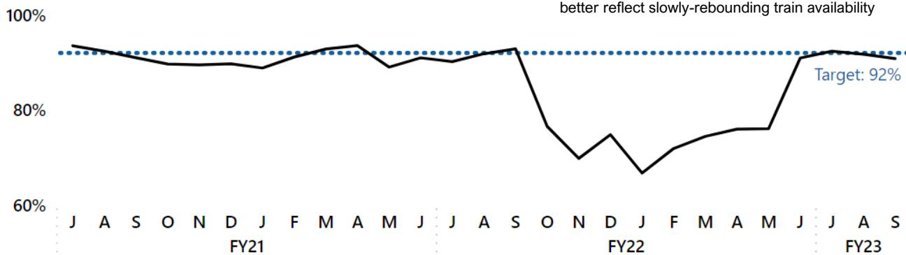
Unplanned service disruptions lowered on-time performance by about 6.4 percentage points during Q1. Common causes of delay include Metro Transit Police responses to customer incidents, breakdowns of rail vehicles, switch or track circuit failures, or track issues. Midday, late night, and weekend single-tracking or shutdowns for planned maintenance lowered on-time performance by about 1.6 percentage points. Through Q1 of FY23, planned delays mainly occurred on Red, Green, and Yellow lines.
