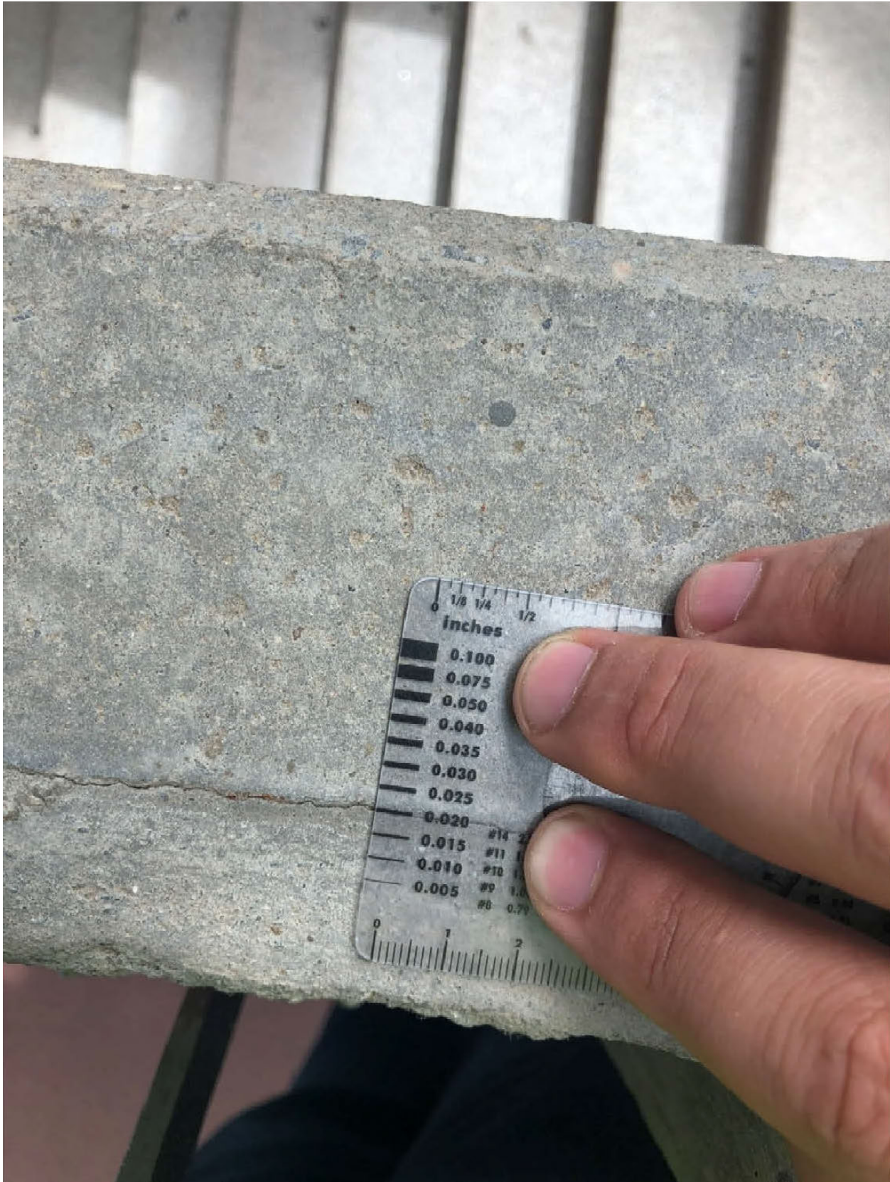
Figure 45: Crack at top face of Panel WP-1235. Source: DeSimone
