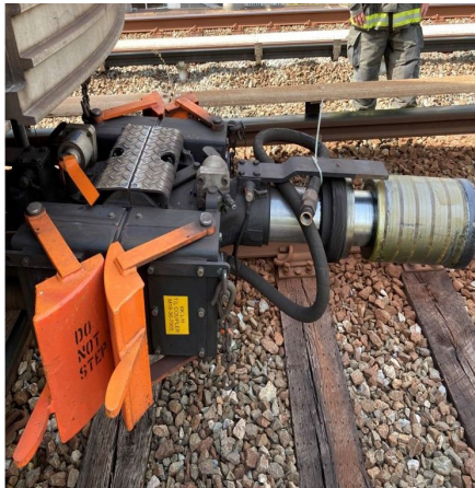
Close up of Car 6079 Front Coupler assembly coupled to half of car 6075 Front Coupler
