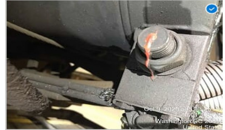
Torque stripe when the buffer tube was installed in car 6075
