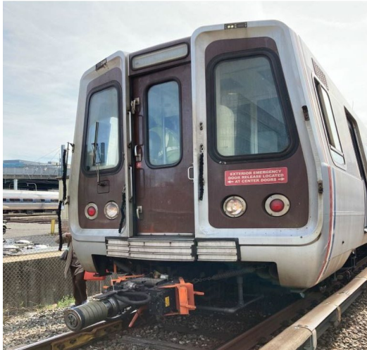
Car 6079 Front Coupler assembly coupled to half of car 6075 Front Coupler
