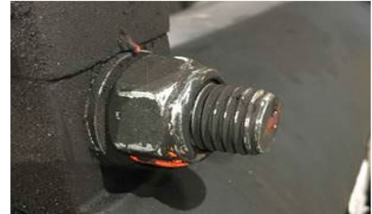
Torque stripe when the buffer tube was delivered to the MRO Shop
