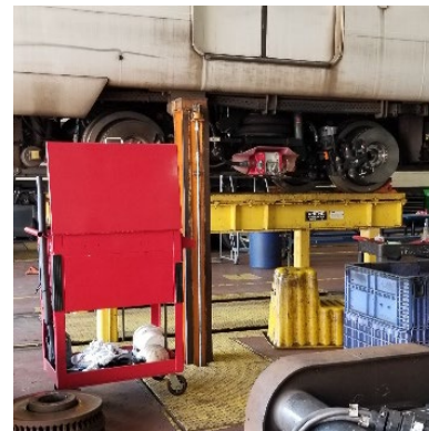
Lifts with Body Jacks Fully Extended
