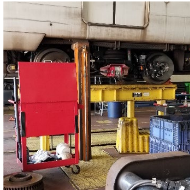
Lifts with Body Jacks Fully Extended
