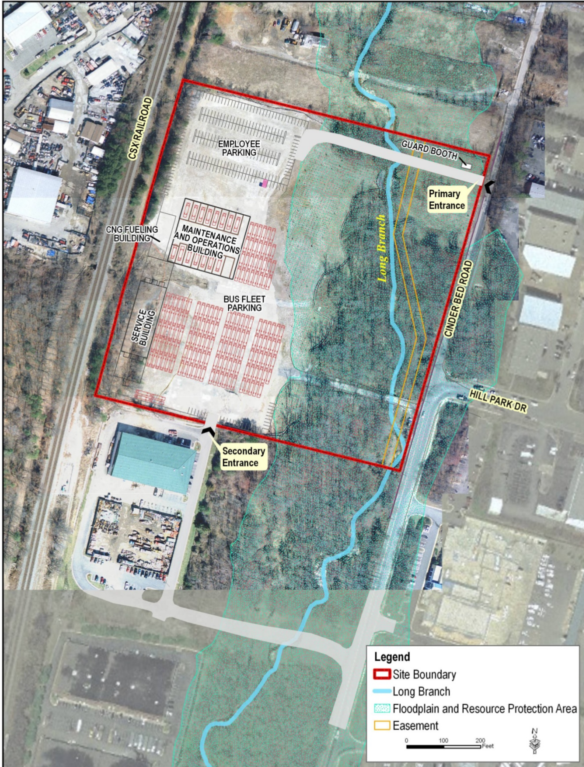
Figure 2: Design Option 1 for Proposed Cinder Bed Road Bus Operations and Maintenance Facility
