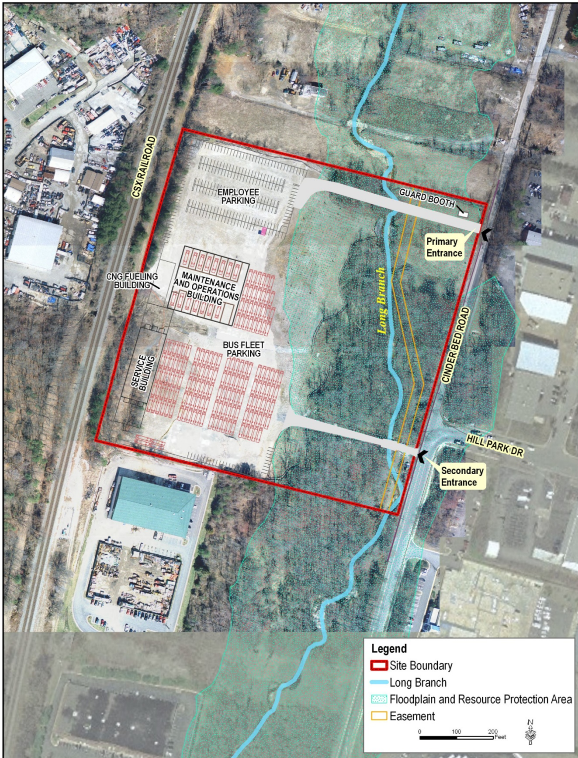
Figure 3: Design Option 2 for Proposed Cinder Bed Road Bus Operations and Maintenance Facility
