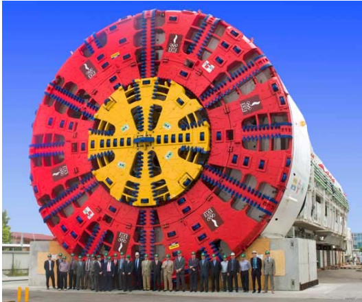
Figure 6. This photo demonstrates the size of the boring machine. The machine takes the place of many hundreds of workers building an aerial structure. Only a small number of workmen are required to keep the boring machine moving.
