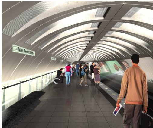
Figure 4. Upper Level Platform is designed in the tradition of the Washington Metro but with lighter tile flooring, contemporary glass railings and projected images on the train room walls. The platform is the same size as the downtown Metro platforms and is actually larger due to the lack of vertical circulation on the platform.
