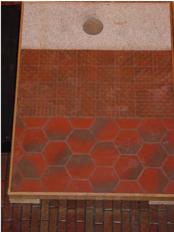
Current 8" hexagonal & 6" Square Truncated quarry tiles.
