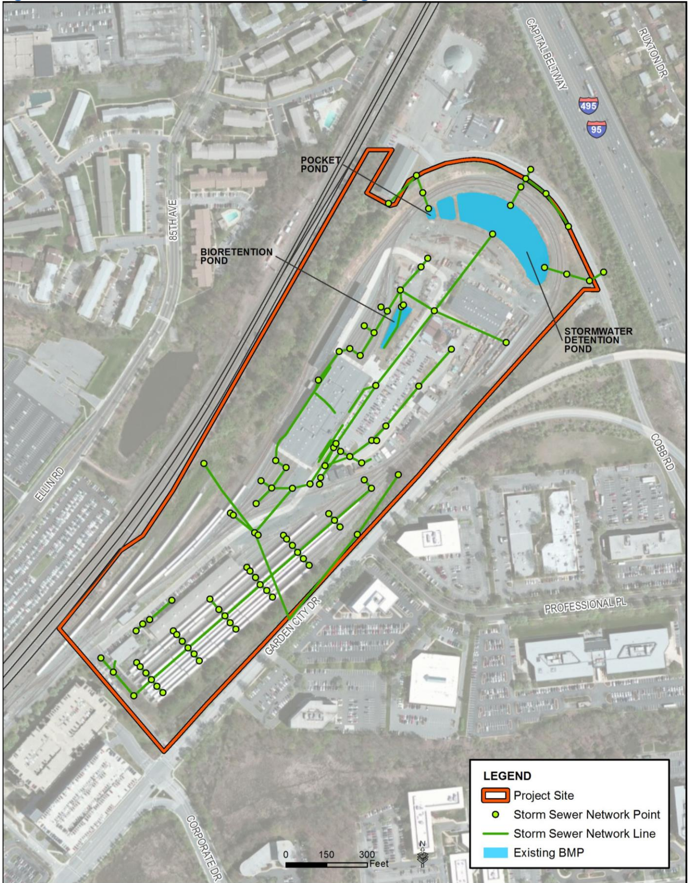
Figure 3-6: New Carrollton Yard Stormwater Management Features
