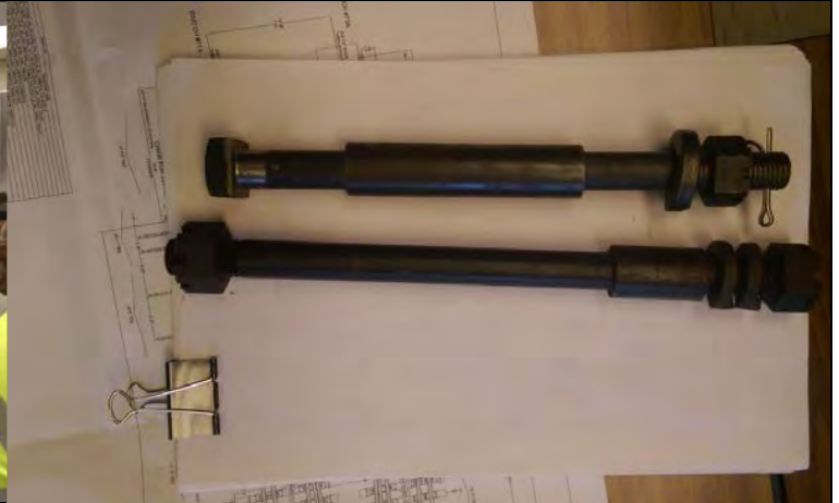
Figure 2: Bolt Comparison of Old vs. New Style (Date: 03/29/17 Time: 0753)
