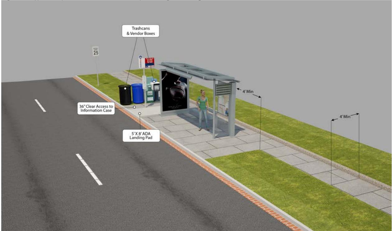
Figure 10: Typical Curb Extension Layout for On-Street Bus Stops Serving Standard 40-foot Bus
