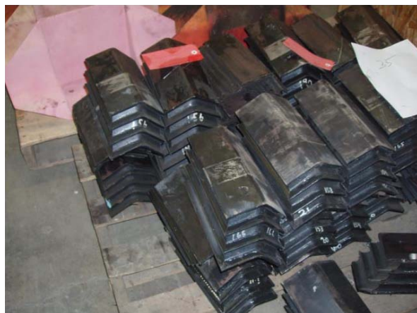
Breda Chevrons Located at TTA Plant in Hornell, NY
