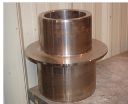
A center pin ready to be installed in a railcar in Hornell, NY
