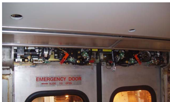
Door Components of Railcar 3129 on Production Line in Hornell, NY
