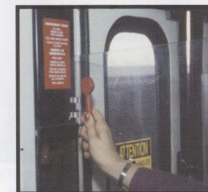
...to break the glass and access the manual door opener.
