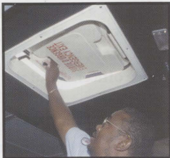
Use the ceiling escape hatch if the doors and windows are blocked.
