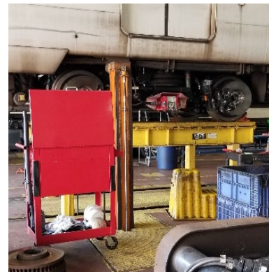
Lifts with Body Jacks Fully Extended
